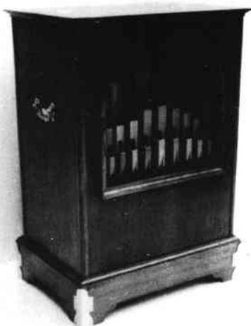
The picture is of organ number Two. Pipework consists of one rank of Stopped Diapasons plus a register. 29 Pipes in total. The register can be manually or automatically controlled. It plays with and one octave higher than, the normal melody. Pipes are voiced at 6ins. W.G. which gives a mellow tone with ample volume. The sound range in still air is about 200 yards.
