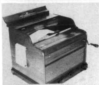
Peerless organette with endless band in place. The small metal roller for keeping the band taut can be seen fitted within the outside loop. This particular roller has the remains of a label which I believe originally carried the legend, "Patent No 16, 748". I have yet to see a roller with legible figures on it. When a long band that hangs below the bottom of the case is played, the organ must be stood on the edge of a table for playing so that the loop can hang clear below both organ and table edge. See Music Box Vol 9, p 118.
