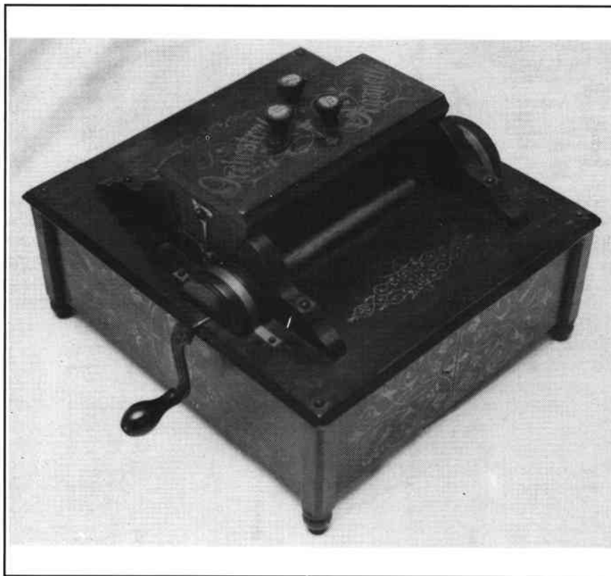
A 14 note, 28 reed, "Orchestral Organette". The reed block and stop arrangement on this instrument was the subject of Joseph Mark Drapers only successful patent application, no 12,670, on 19th September 1887.
