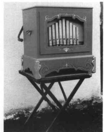
The 20-note pipe organ, built on the lines of the Hofbauer type.
