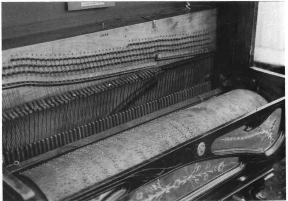
The 48-note piano has 20 additional hardwood hammers, which can be seen to the right-hand end of the barrel, giving a mandolin effect.
