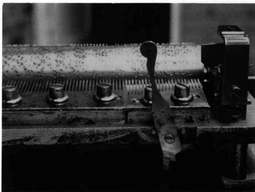
Typical ON/OFF lever for Conchon Harpe Éolienne box no 7220, here shown in the ON position against the left hand stop. The lower end of the lever is a cam pressing down the sprung bar which is pivoted under the bedplate and has lifted the zither to touch the comb teeth.
