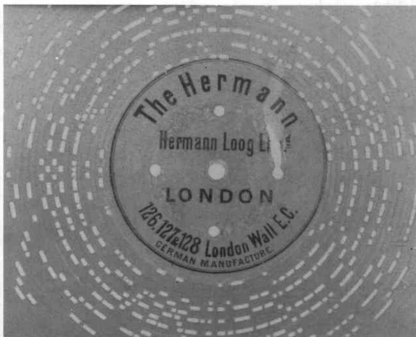
Fig. 8. The underside of a well played Ariston disc showing Loog's way of customising the discs for his Hermann, the disc is otherwise standard, this particular one being No 1. Rule Britannia.
