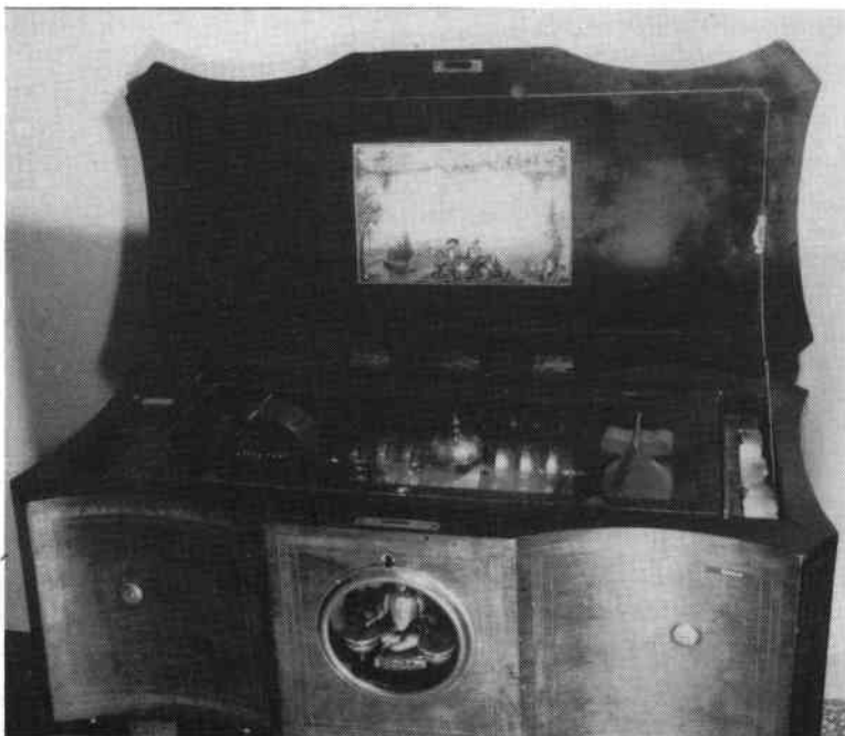
Fig. 3. Bremond 8873, 42cm cylinder, 8 airs, with automaton of man turning his head and striking the drums. The BAB stamped on the governor cock is the same as on serial no 6329 (page 303 of Vol 11) but with lyre added. The lyre adorned most Bremond tune sheets.
