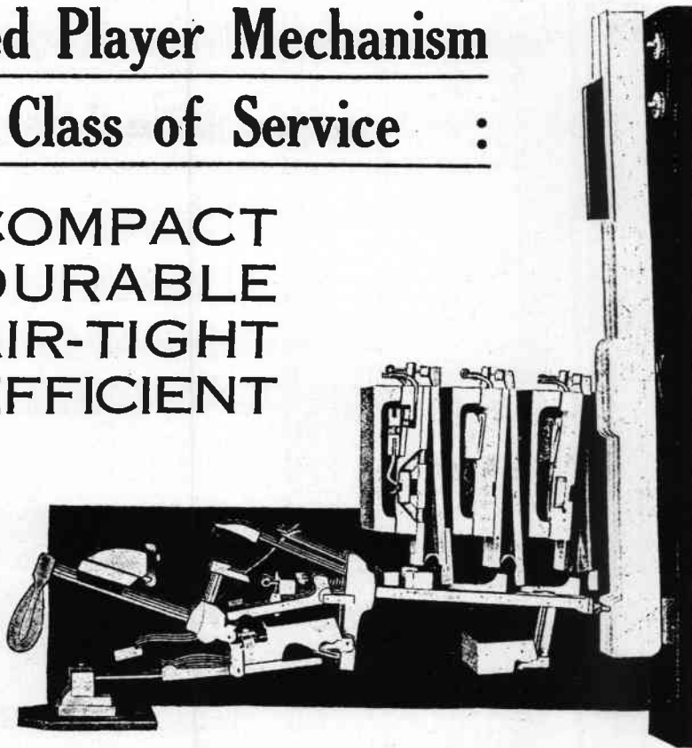
Section through Pneumatic Stack : Schulz Player Mechanism.
