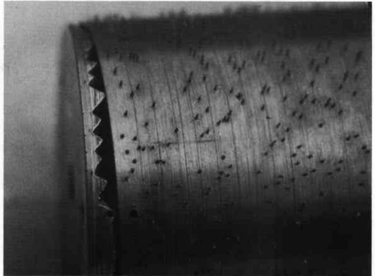
Bass end of 22386 cylinder dismantled for re-pinning. Note small nicks filed on end cap to indicate where notches were needed to clear cylinder pins. Pinning was taken closer than usual to the edge of the cylinder.
