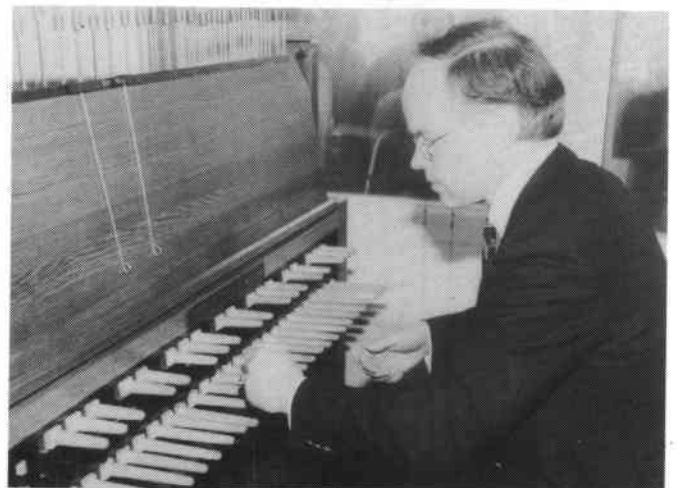
A heart rendering rendition of "Rule Britannia" being thumped out (literally) by Dr. Haspels at the Carillon's keyboard. The vertical linkages connect direct to the bell hammers.
