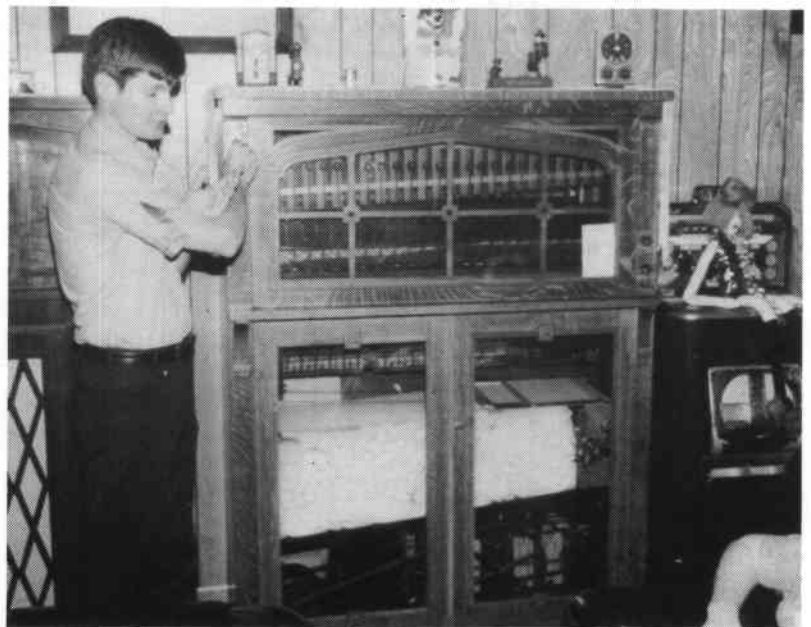
Our host at Rudy Edward's collection, demonstrates a Link 2-E coin piano with mandolin and xylophone. Note the endless paper music roll!
