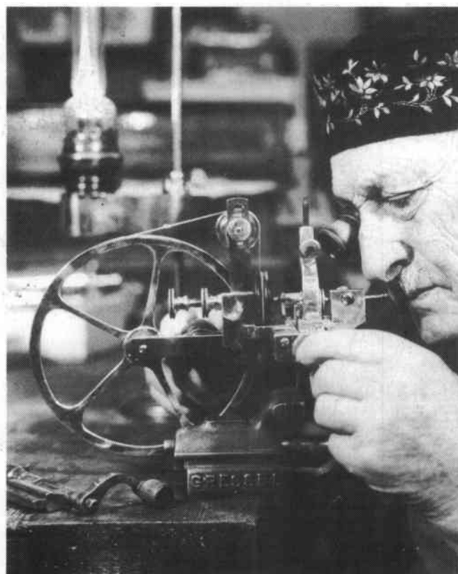
Balancing the wheels of the governor assembly on a special machine.
