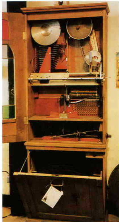
Kilkhampton, Gramophone volume control. A plunger blocks the horn.
