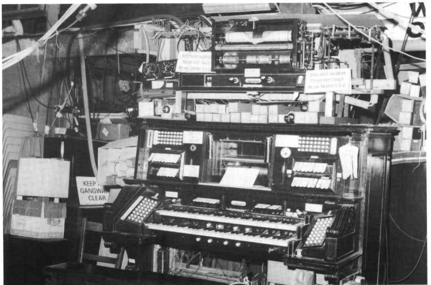
Frank's 18 rank Aeolian pipe organ with a Duo-Art-organ roll playing attachment wired in above.
