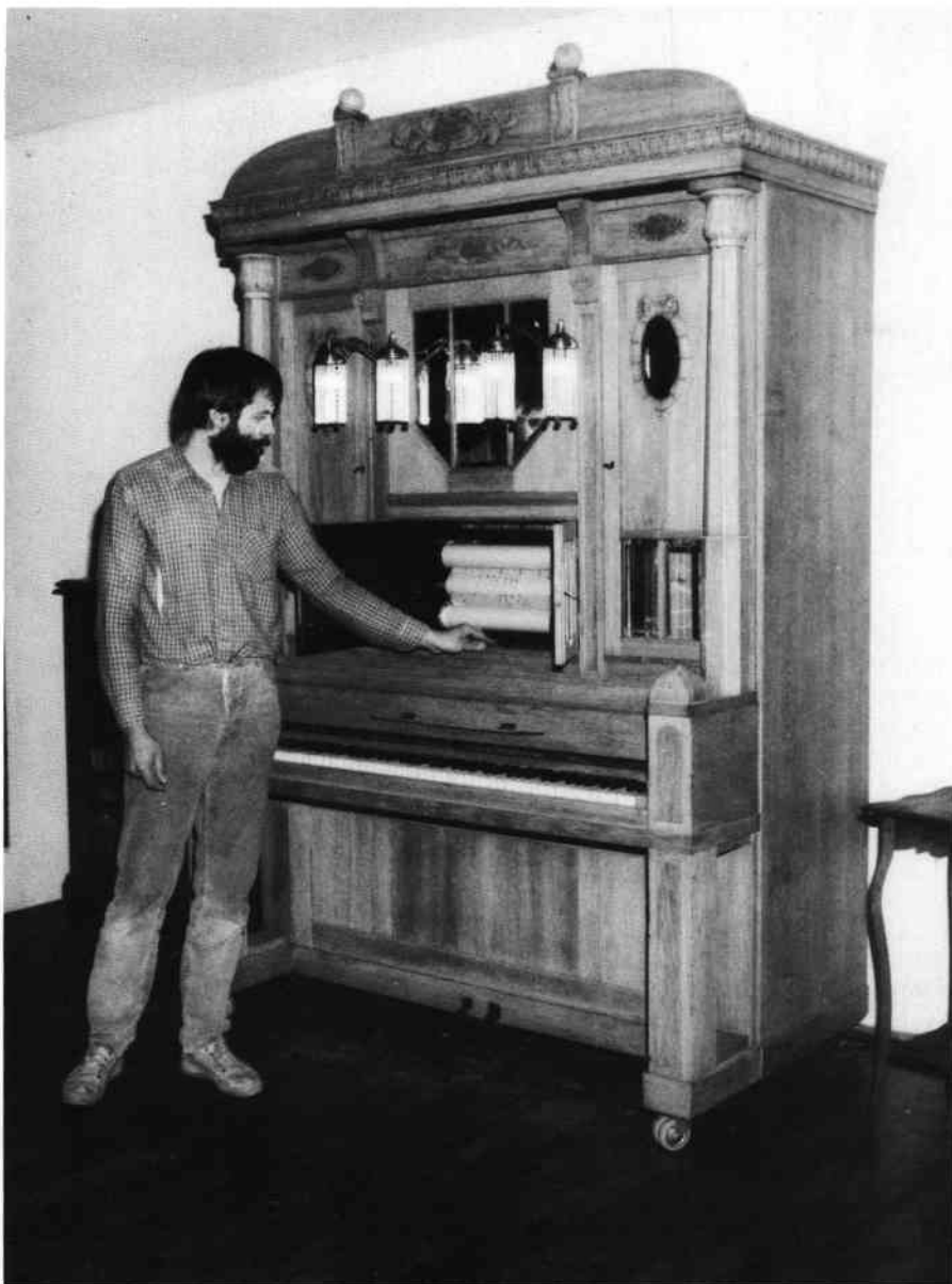
Thomas Janssen plays the most popular Lösche instrument made. An orchestrion with flute and violin pipes.
