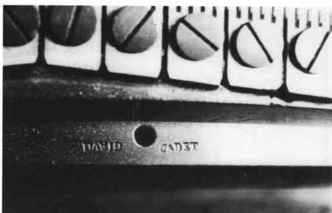
Fig 6: Teeth in groups of five. The hole above DAVID CADET is for the instant stop lever screw below, usually blind.
