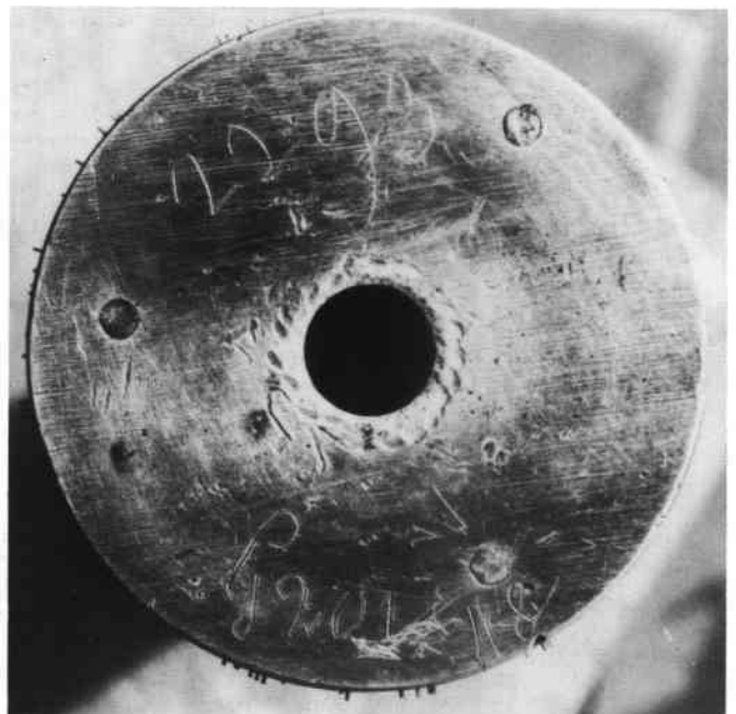
Fig. 3: Typical Langdorff markings on base and cylinder cap, – serial 2293 and G201-48. Where, as here, the bore has been closed in by hammering it is wise to check that the cylinder is still reasonably concentric and the pin tips accurately concentric with the arbor.
