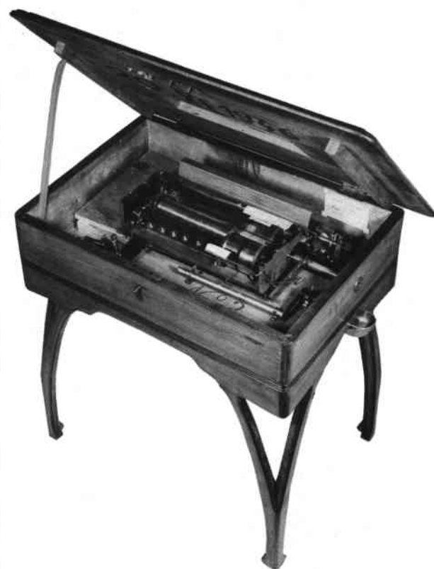
Fig. 2. The winding handle is shown parked inside the table and beyond it the levers for the CLOSED notice and for obstructing the coin slot when run down. The coin mechanism accepted undersize coins without providing any music.
