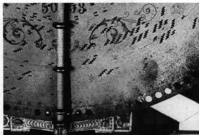
Fig. 8. Part of 19½ Polyphon disc 50253, showing the mandolin effect based on groups of four notes. All these groups play at about six notes per second. The helical angles only vary, in this case from about 42° to 50°, on account of their different distances from disc centre and therefore their different surface speeds.
