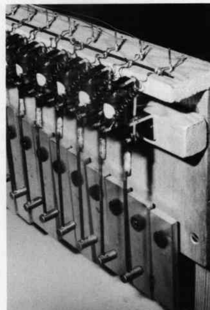
A 20 note Glockenspiel electrically operated, used by Graham Whitehead to demonstrate the advantages and simplicity of an "all-electric" action.
