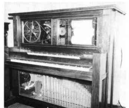
(Above): Reproduco orchestrion, often used in funeral parlours, plays from NOS rolls, similar in width pitch and scale to the standard 88-note, but on different spools and is arranged for organ register.
