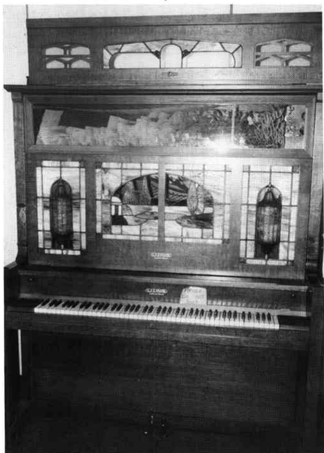
The Link AX orchestrion made by the Link Piano Co. Binghamton, N.Y. plays piano, mandolin, maranbaphone, snare drum, triangle, tom-tom, tambourine and Chinese wood drum. Link pianos were made from 1913-1929 and this example was their largest. Notice the endless paper roll in the top cabinet.
