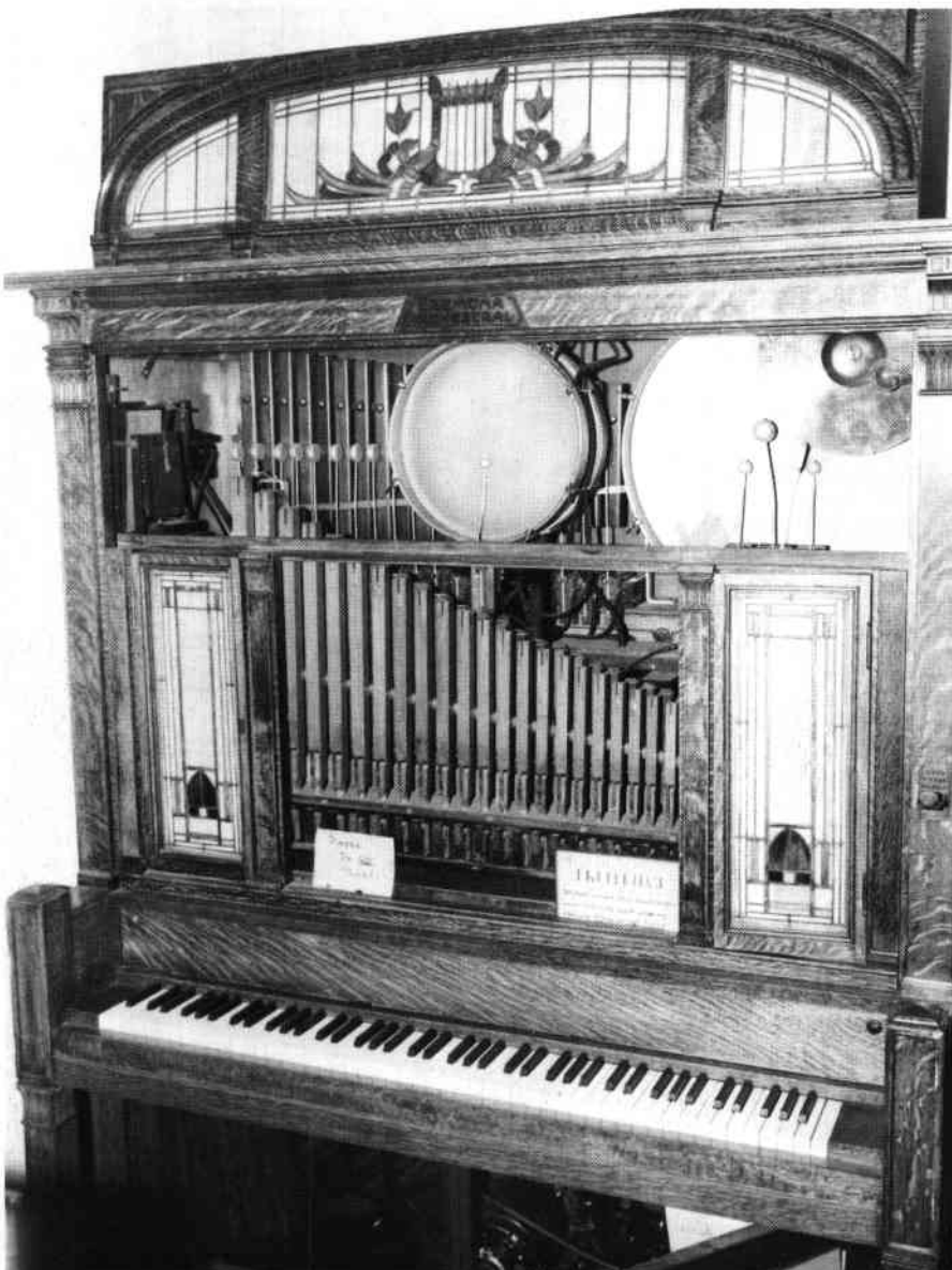
(Left): Cremona "style J" made by the Marquette Piano Co., Chicago. A very rare machine made in 1918 plays 10 different orchestral effects, piano, mandolin, flute pipes, bass and snare drum, cymbal, triangle, xylophone and tympani.
