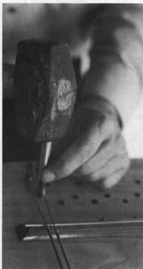
Fig. 10. Hammering the wrist pin home until the turns of the wire are within approximately 4mm from the surface of the wrist plank. It is preferable to use pins of a size larger than the original.
