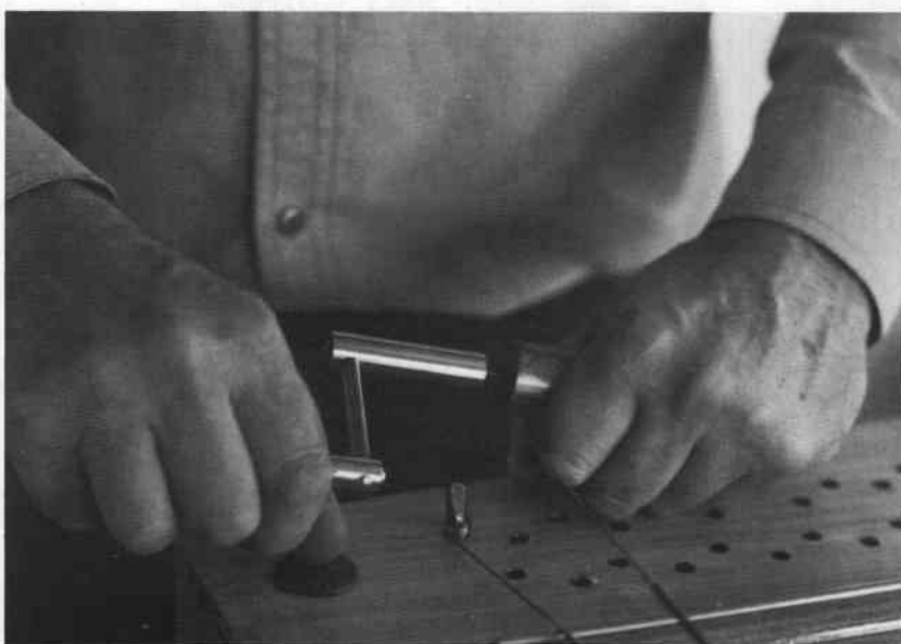
Fig. 8. The piano wire is shown being wound onto the wrist pin.
