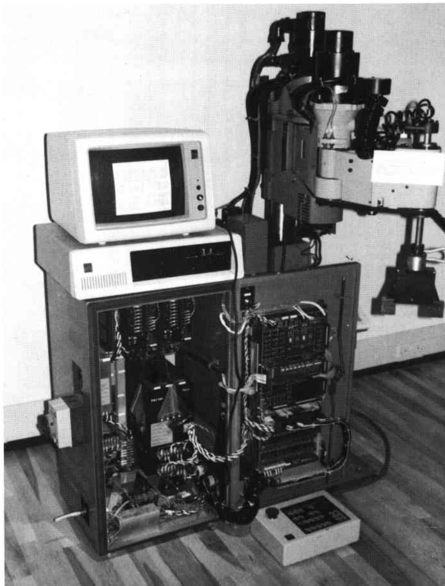
An example of the modern development of old-time automata - the IBM 7535 robot designed to assemble typewriter keys.
