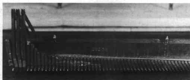
Fig. 7. Comb of serial 38398 with tuning marks, seventeen soldered dampers, and vertical line of dots - a convention for indicating the last tooth needing a damper.
