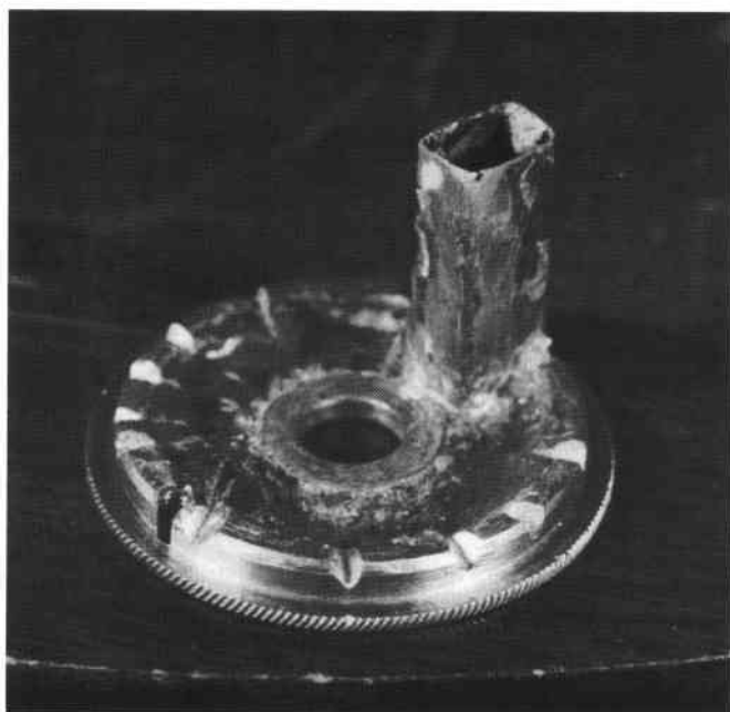
Fig. 4. Treble end cap of serial 38618 showing knurled edge, grooves cut to clear pins near the end of the cylinder, and zinc shield to leave space in the cement for the drive bar. The tapped hole for the snail cam follower is perilously close to the cylinder.
