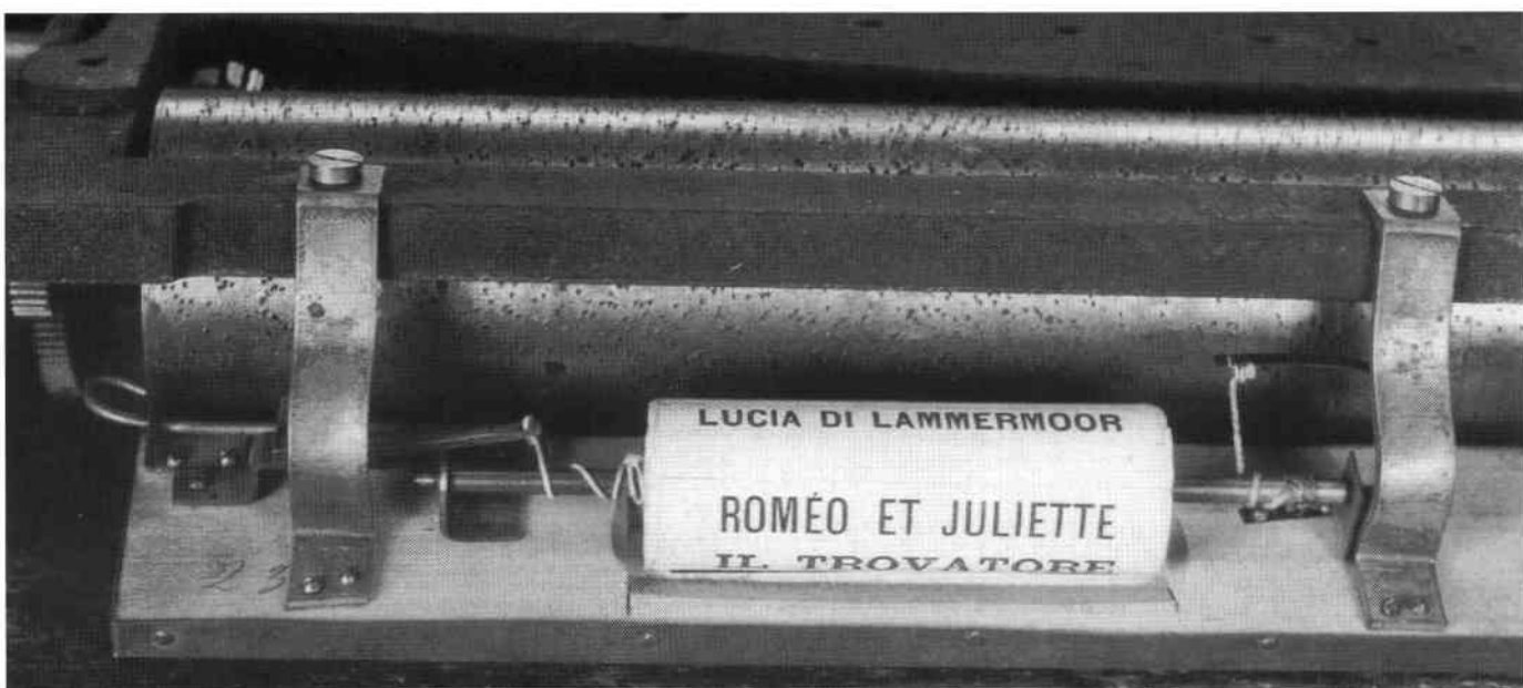
Fig. 9. As the cylinder shifts towards the bass end the operating rod pulls the short arm of the spring bracket causing the long arm to lift and pull the cord which turns the display drum to the next tune. Tension on the leaf spring seen at the right is thereby increased, ready to turn back the drum after tune 8.
