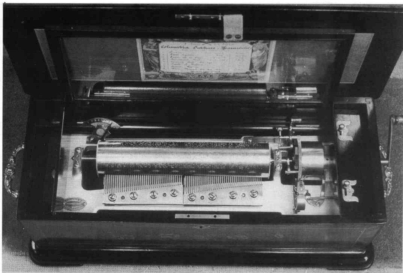
Fig. 7. Paillard "Columbia" serial 96998, eight airs, with PVF tune sheet and oval plate at left front of bedplate embossed C. Paillard & Co./Manufacturers/Ste. Croix Switzerland. Some later bedplates had cast lettering in the same position reading USA/PATENT/SEPT 25th/1894. The stub axle engaging the snail cam carries a fork which is driven from a peg on the spring barrel, as shown.
