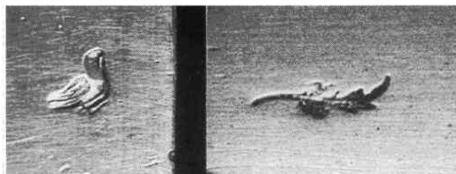
Fig. 5. Craft marks: 5mm bird on bedplate of Lecoultre 27740 (which also has the "rampant puppy"); and 6mm leaf on the governor block of C. Paillard 2699 (which also has the 4mm square C/P/&C on the governor cock).
