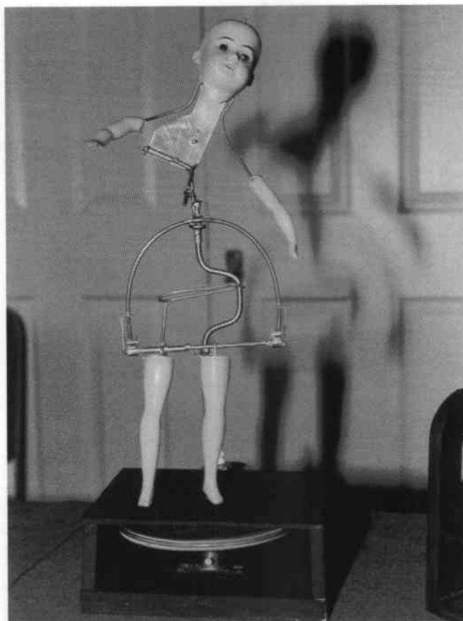
Modelled on the ingenious design by Decamps, Lyn's model demonstrates how to achieve the maximum of movement without any cams at all.
