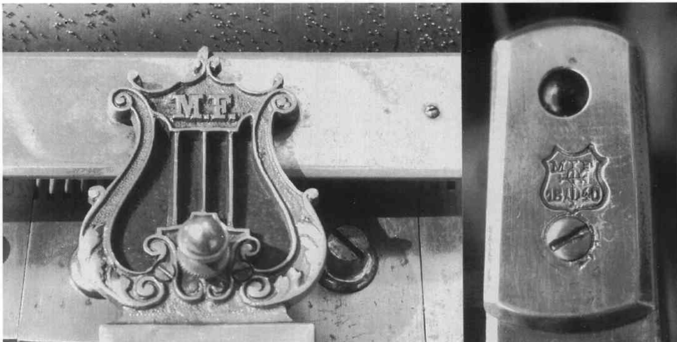
Fig. 8. Mermod Frères markings on zither and governor cock.
