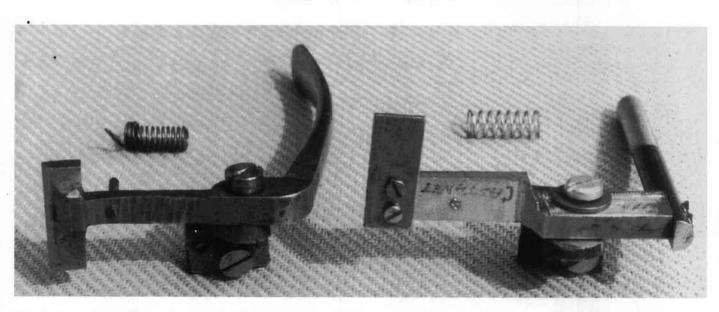
Fig. 8. Conventional cast brass on/off lever with bearing bracket and spring. Note stretching marks made during adjustment. Beside it, a 3-piece replacement as fitted to serial 1917.
