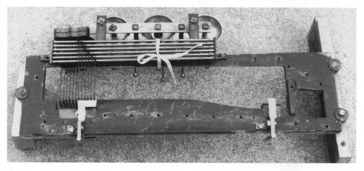
Fig. 9. As chalked by its maker under the comb area, here is serial 1917 bedplate inverted and screwed to blocks for safe support. Tape secures the six bell striker rods, their new on/off lever is fitted.
