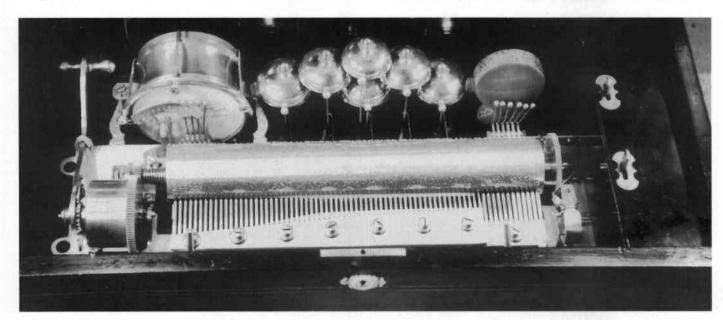
Fig. 5. Serial 1917, 13" cylinder, ten airs, drum, bells and castanet.
