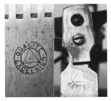
Fig. 3. Ullmann trade mark on main comb and governor cock of serial 1917, made about 1891.
