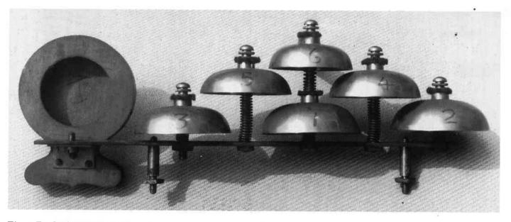
Fig. 6. Back view of the bells and castanet gantry with bells numbered in pitch order, lowest No. 1. Bell 5 needs lowering, it is dangerously close to bell 6.
