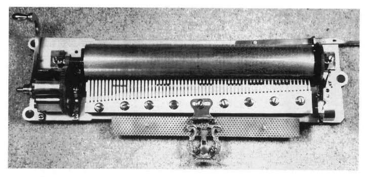
Fig. 7. Zither moved to show the six groups of 4 teeth on serial 1681 comb. The second and third groups from the bass end are a teeth, 440 and 880Hz.
