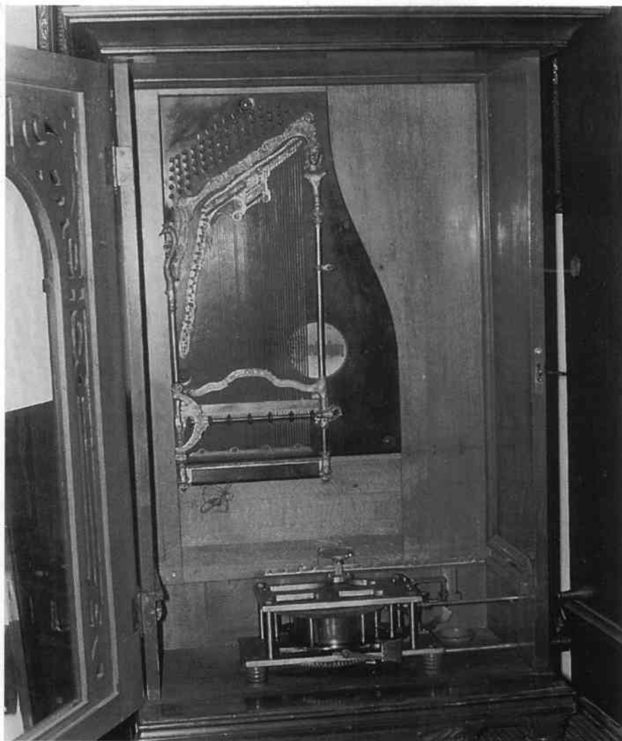
Fig. 5. With the disc removed, the shape of the harp is revealed together with the detail of the finely-finished frame for the strung back.
