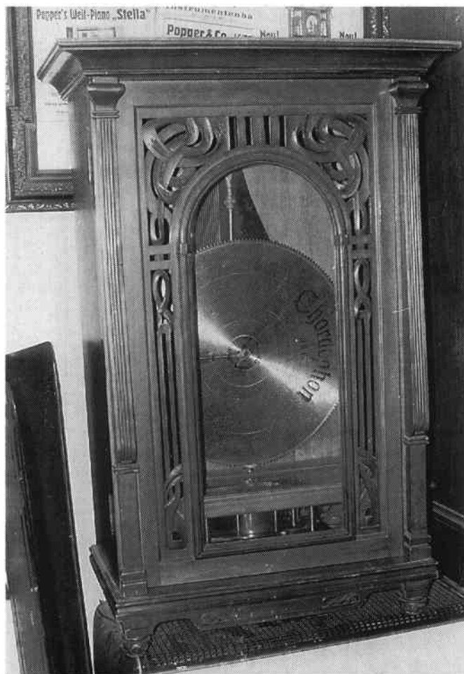
Fig. 3. From the collection of Werner Baus comes this fine example of the upright-cased model playing 60 notes using a disc 19 \frac{3}{4} -inches (50cm) in diameter. The case design is clearly after the jugendstil fashion.
