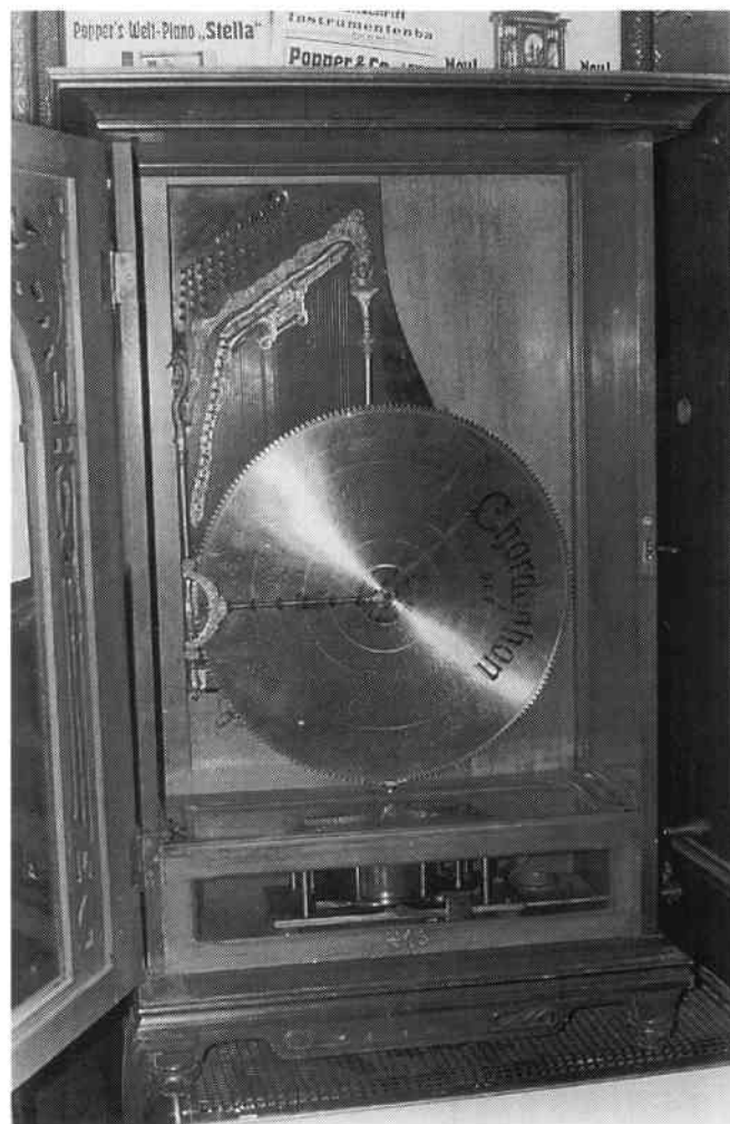
Fig. 4. Interior view showing the disc in place and also the slim proportions of the motor assembly.
