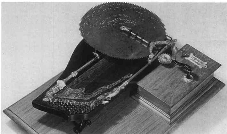
Fig. 2. This is another variant on the 30-note style. The clockwork motor, now provided with a better winding handle and coin-operated, still appears as an extra item. In this picture, the disc is not in contact with its drive pinion due to misalignment of the motor assembly. The notice on the coin-slot reads Einwurf 10 Heller suggesting that this example was made for use in Switzerland.
