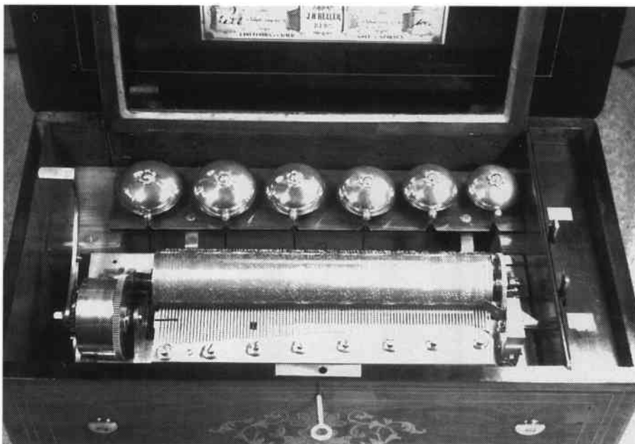
Fig. 2. Serial 1076, with marked a teeth (440Hz) and bell teeth. The bells are plain, with plain ball strikers, and cannot be switched off. Small Heller labels numbered 2 and 3 are stuck beside the control levers. The governor fly is not sprung (compensated) as claimed on the tune sheet.
