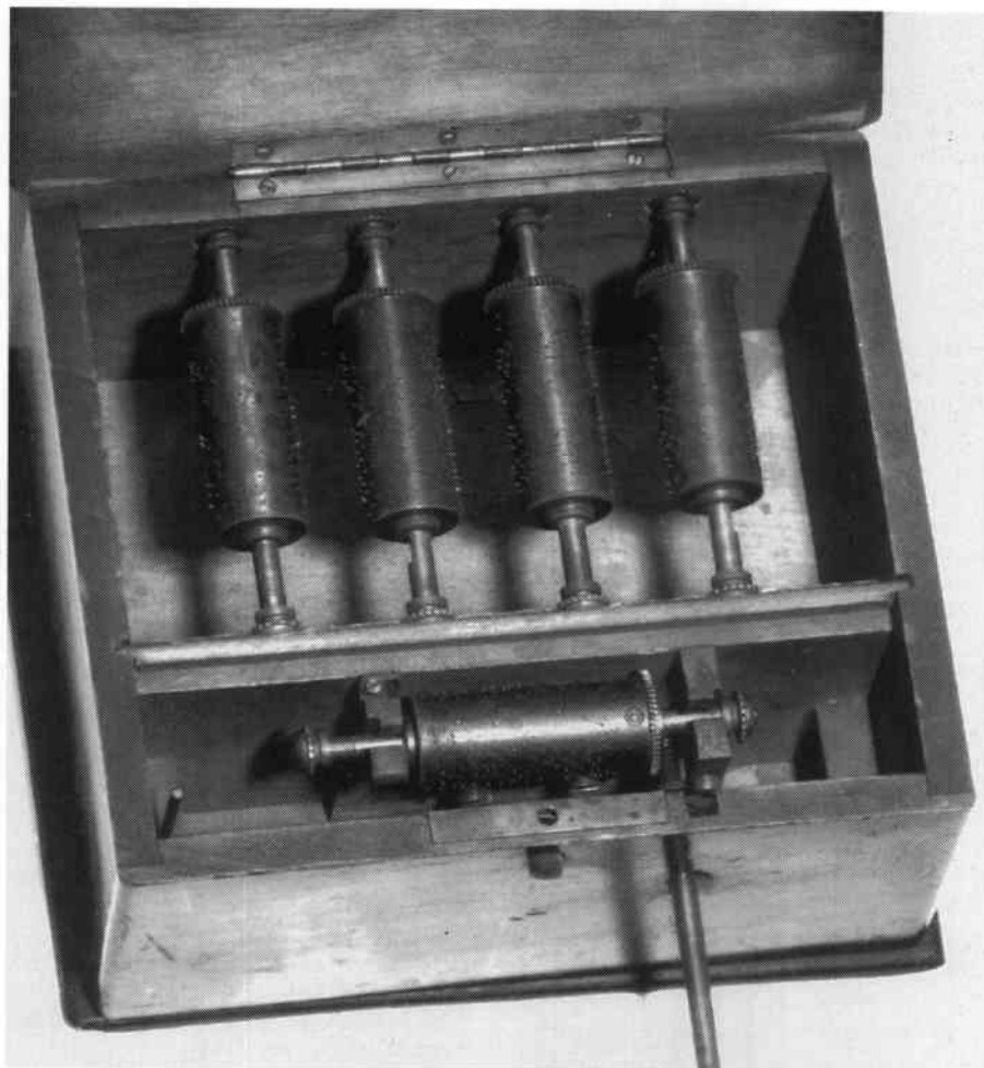
Fig. 11. Hand-cranked "Multiphone" with cylinders 3\frac{1}{4} inch long including gear and spindles. (Not to be confused with the 24-air coin-slot 1905 phonograph of the same name!) More details on page 37, MBSI Journal, Spring 1986.
