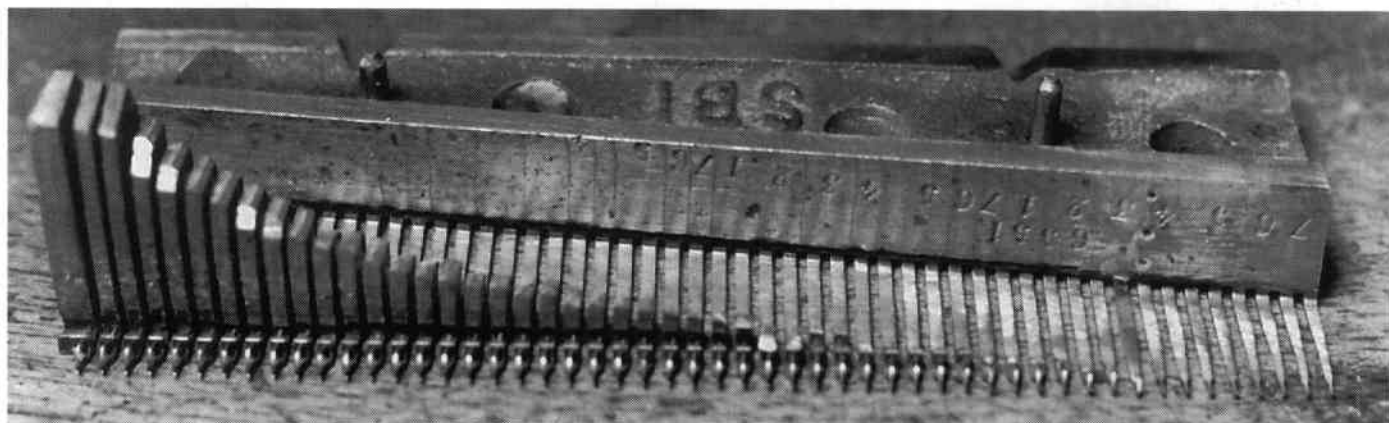
Fig. 6. Bass comb showing foundry cast SBI and stamped serial number and pitch numbers. The a teeth are numbered 4, semi-tones not numbered. The line of three dots marks the end of dampers; there are 7 soldered dampers.
