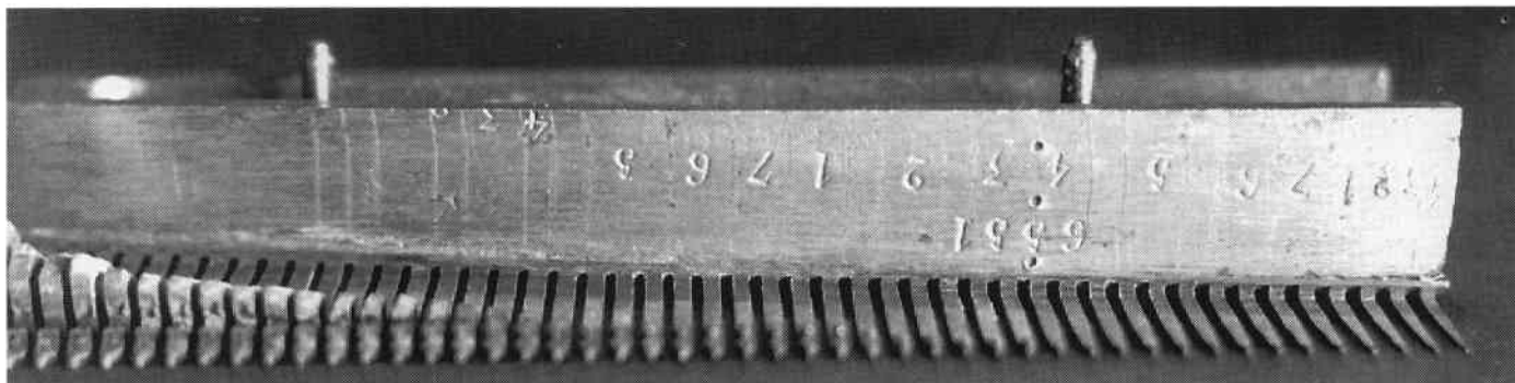
Fig. 7. Same markings on serial 6551 treble comb. Again no feather dampers but 6 soldered dampers.
