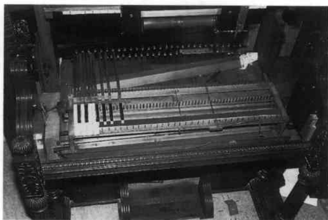
Keyboard of 29105, showing the pneumatics at top and wire 'pull-ups' acting on back of elongated keys.
