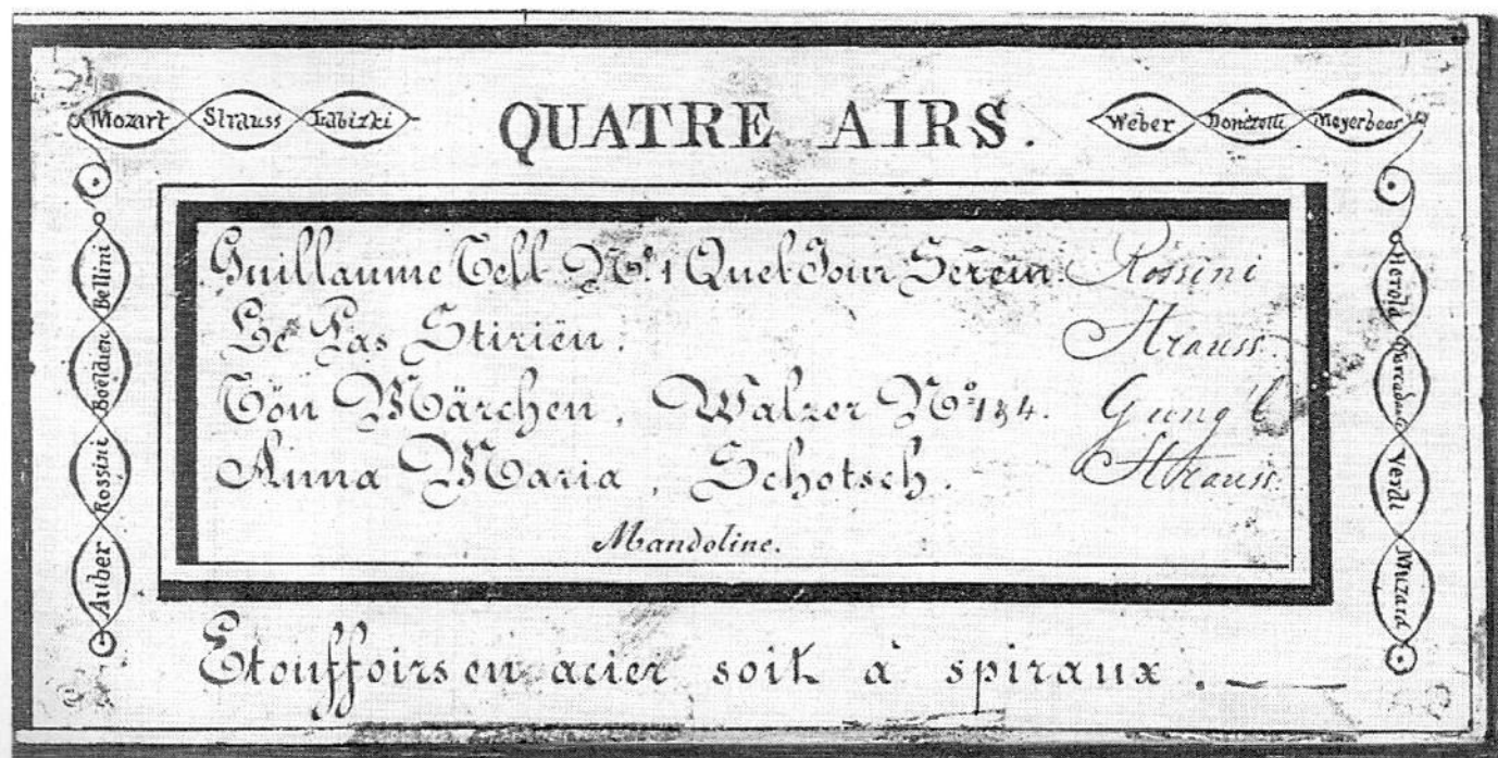
Fig. 11. Tune sheet of Langdorff 10380, in black on buff card 6"x 3" (152 by 76mm). The 13" (33cm) cylinder plays 190 comb teeth. The bass end cylinder cap is scribed G616/57 for gamme 616 made in 1857.
