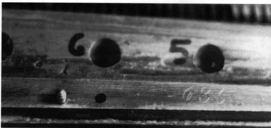
Fig. 12. Extra dowel between nos. 6 and 7 of the eleven comb screws. Scribed 635, and cast number 12 just seen between the dowel and my figure 6.
