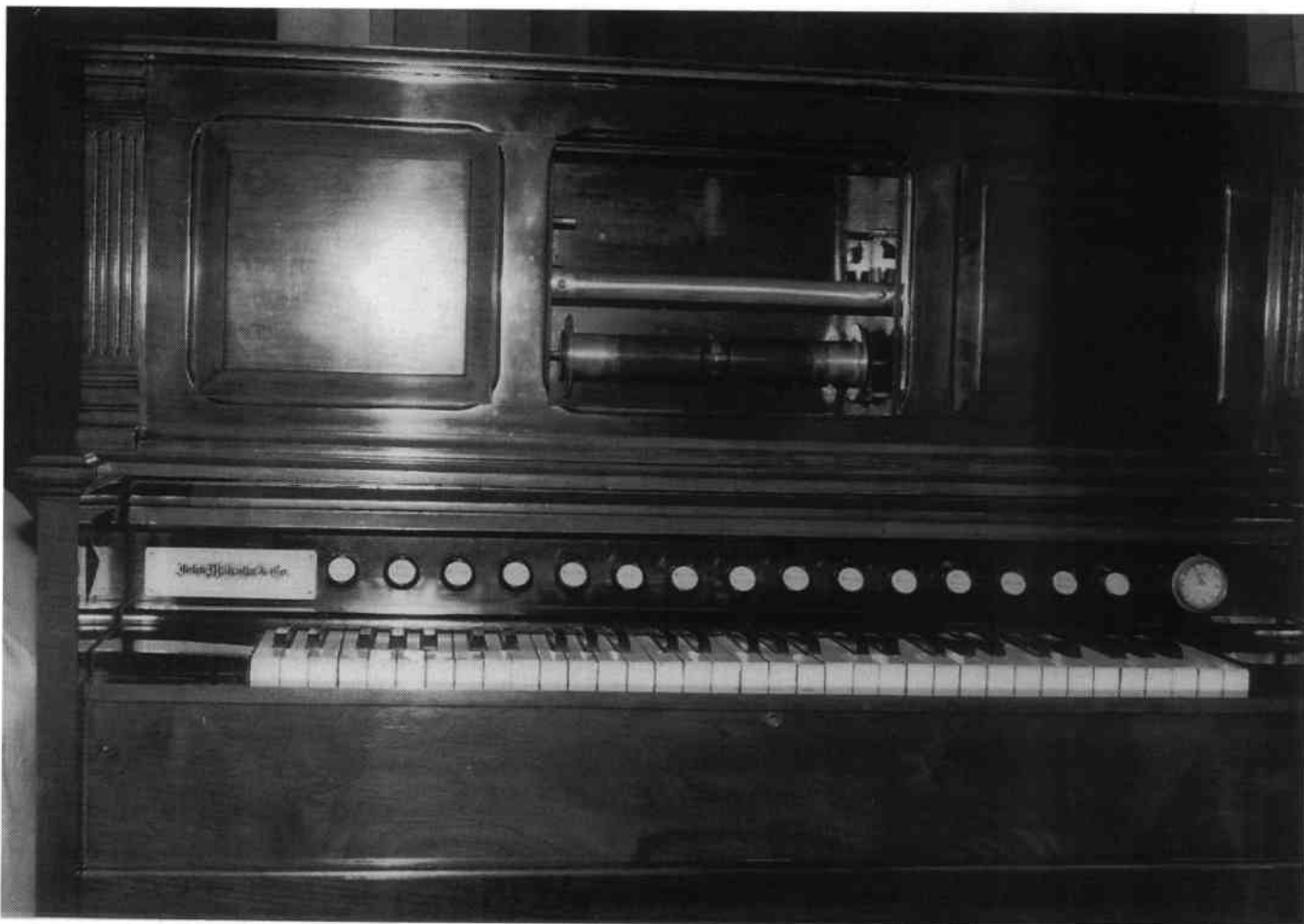
Fig. 3. Closer view showing 65/58 adaptor in spool box and no holes in panel under keys to let sound out.
