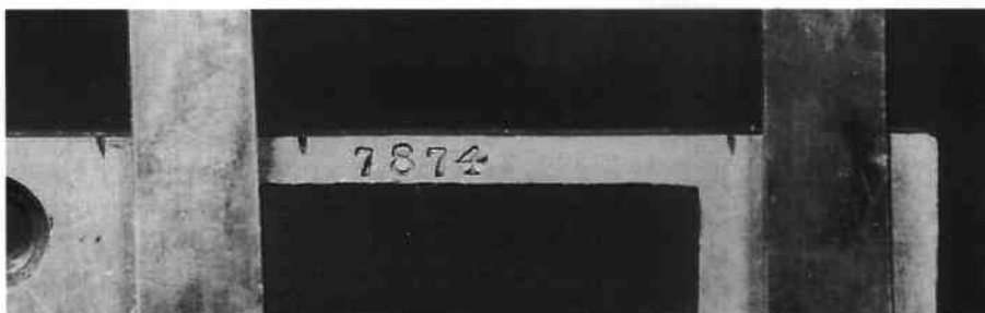
Fig. 5. Mystery 7874 stamped under Lecoultrre bedplate. The nicks filed at the edge indicate the travel of the control levers.
