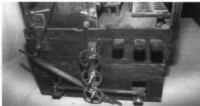
The length of the stroke on the feeders could be adjusted by this very well made rack.
