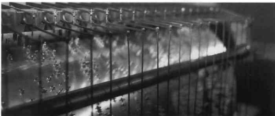
The clevis joints at the back end of the keys on the key frame.
