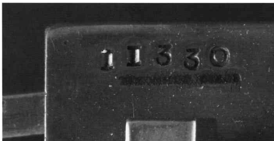
Fig. 6. Ducommun Girod literally stamped out from the bedplate of serial 11330 - key-wind, 6 air 10½" (265mm) cylinder, made about 1836.
