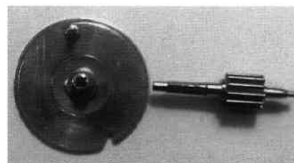
Fig. 2. Disk with pinion, responsible for the rotation of the cylinder.
