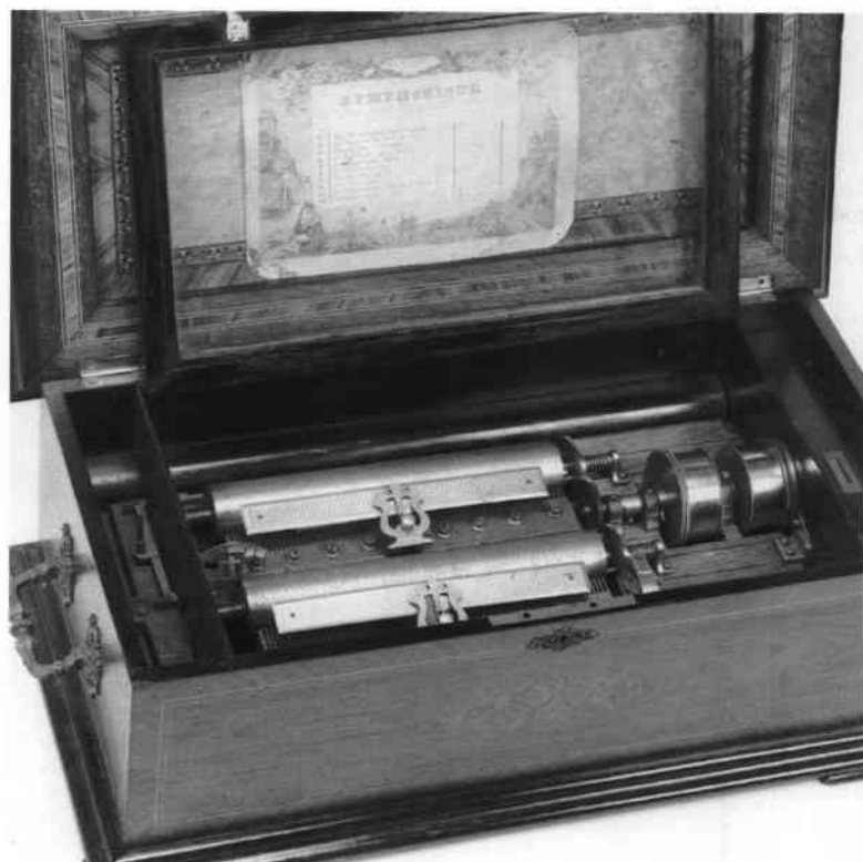
Fig.8 Cuendet Duplex 20867 with change/repeat lever in bass end partition. Front cylinder operates tune indicator and its great wheel, doubling as drive gear, also drives the governor. Probably made about 1895. Photo thanks to Christie's.
