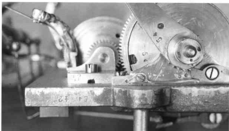
Fig.4 Blank number 54 on the bedplate edge and four spring components all with matching undersized figure 4. Blank number 42 has normal figure 4. The tail of the bell lever can be seen under the bedplate, in "bells on" position.
