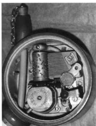
Above: The flat, weighted disc pendulum engaged or frees the butterfly in this MELPA, Switzerland musical movement. The c.1950 18-tooth movement has an aluminium cylinder and plays "Lieber Augustine".
