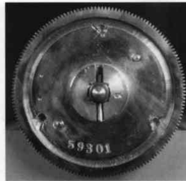
Fig.9. Great wheel with three chamfered-exit stop slots. Gamme 4982 is scribed on the bass lead, cylinder cap and white metal comb base.
