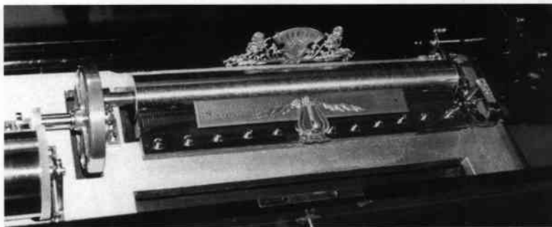
Fig.4. Serial 49539 with large double springs and internal gear drive to cylinder, allowing 60 minutes continuous play.
