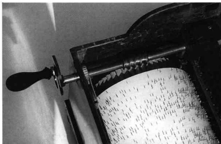
Fig.1. Corner blocks for additional strength. Extra ratchet and pawl for safety.
