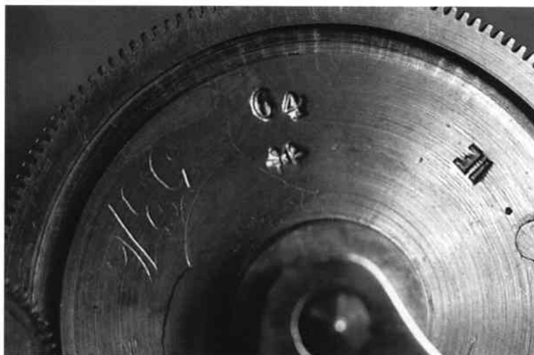
Fig. 3. Rivenc 28844 great wheel, scribed gamme 5316 and stamped 64 the blank number of the cylinder assembly, also the "asterisk" and the non-serif IE.
