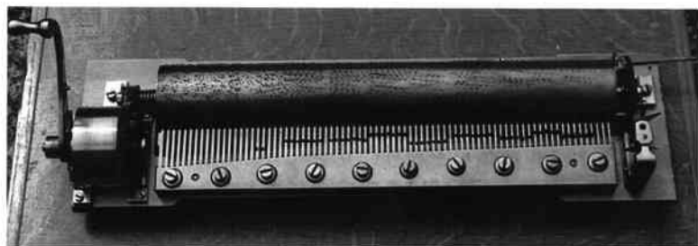
Fig. 2. Rivenc 28844 with the comb marked for the two 440Hz a teeth and the eight groups. Corresponding helical lines of pins can be seen on the cylinder.
