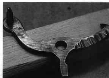
Fig. 4. The Rivenc 28844 stop arm. It has been vigorously stretched to curve the right side upwards and thereby lift the catch closer to the stop tail.
