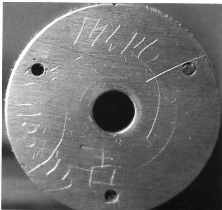
Fig. 10. Bass end cylinder cap scribed 21741, 1105, and the craft mark. The three holes are for pushing out the brass pegs fixing the barrel to the end cap.
