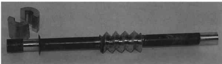
Fig.8. Worm soldered up. Outer bearing ready to solder and turn to size.
