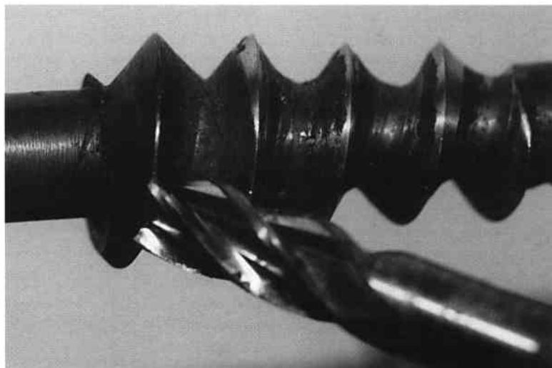
Fig.6. The worn worm. Setting the end mill for alignment.
