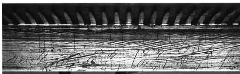
Fig. 3. Part of the comb base, - the treble end is at the left of the picture. The small groups of teeth scribed below the serial number 30813 are 3 fa , 3 sol , and 2 fa . Between each group there is one tooth tuned to the semitone and marked with a pair of short sloping lines.
