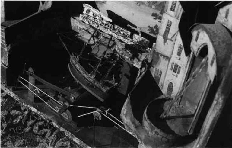
Fig.2 Close-up of the rolling ship, train and musical box drive arrangement.
