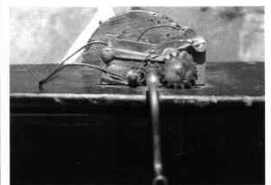
Fig. 3 Side view showing casting and gear work of paper transporting mechanism. Note the roller before tracker bar to keep music roll airtight on holes.
