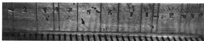
Fig. 4. Part of 29254 comb with pitch lines and numbers, and groups of up to four teeth. The figure 1 on its side signifies f ( ut ) sharp.
