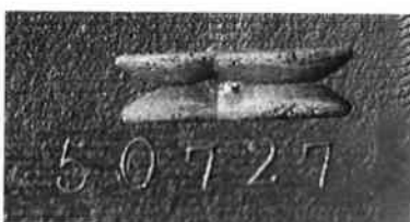
Fig. 6. Serial number on the planed cast iron bedplate just below the double slot for the peg on the tune change lever.
