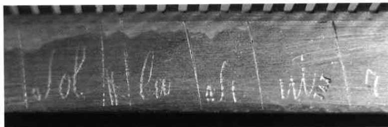
Fig. 3. Piano comb of 40746, bass end at left (because it is upside down), with JAJ stamp in the ut group of 4 teeth.
