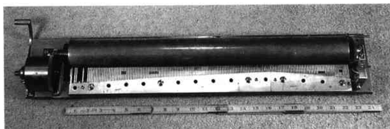
Fig. 2. Nicole 40746 with their usual forte piano comb arrangement. Marked teeth are a, 440 and 880Hz.
