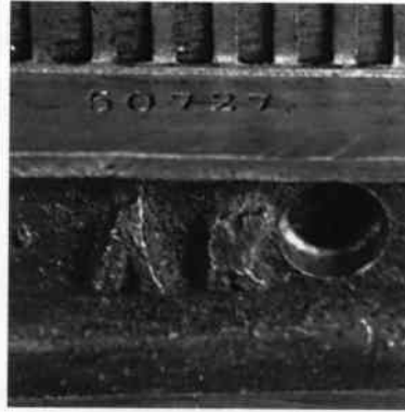
Fig. 7. Cast AK and stamped 50727 on comb base.
