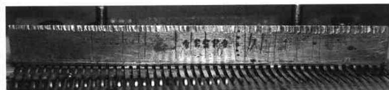
Fig. 4. Harp comb of 43534, showing the whole front length of the comb base stretched, more severely at the treble end. Every pitch change is scribed, with sol fa notation.
