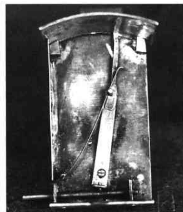
Fig. 16. Back view of tune indicator. A pin on the push rod actuates the lever which is kept in contact with the pin (and thereby in contact with the cylinder) by the leaf spring.
