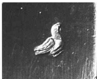
Fig. 10. Bird craft mark, 5mm square, at right back corner of brass bedplate.
