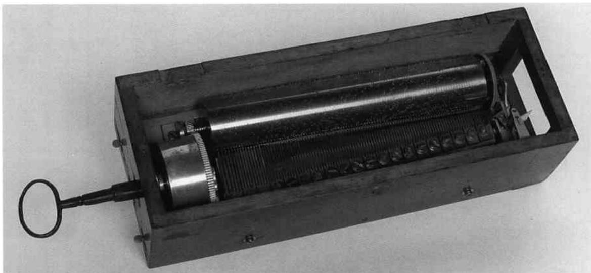
Fig. 1. An early key-wind box with 20 part sectional comb.
