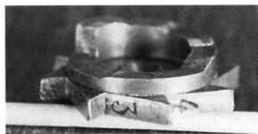
Fig. 3. Snail cam with numbered steps, and step 4 deleted leaving tune 3 to play twice.
