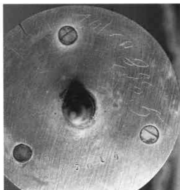
Fig. 11. Cylinder end cap with stamped 7019 and scribed gamme number G 358. The three holes, plugged for centrifuging, allow access for pushing out the three pins fixing cylinder to endcap, which had to be done to insert cement after pinning.
