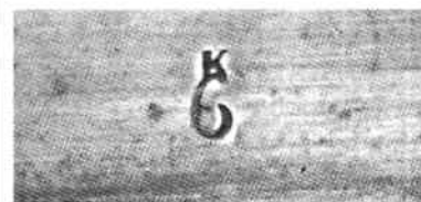
Fig. 4. The K perhaps came with the casting, and the 6 probably added when assembling the blank.
