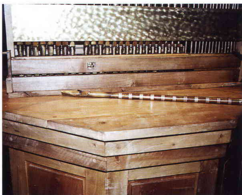
Fig. 5. A replicated pipe. It is directly comparable with a modern pipe, including tuning ears.
