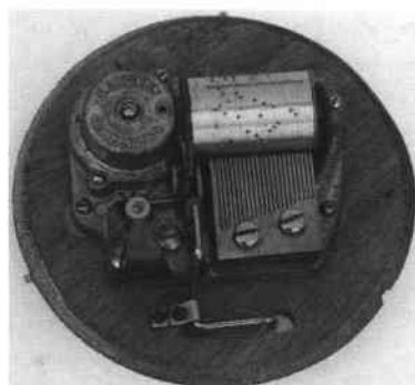
Fig. 6. Lador die cast alloy base and spring case stamped Lador, Switzerland without stop work. Comb as for fig. 5. Nickel-plated cylinder.
