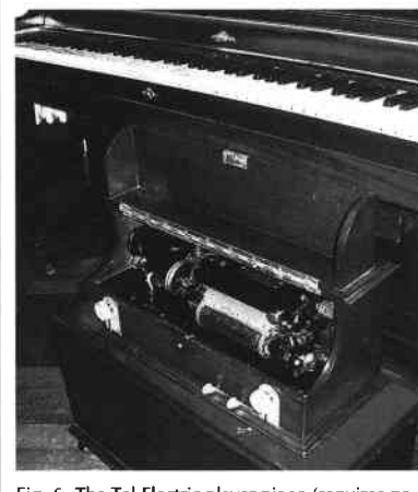
Fig. 6 The Tel-Electric player piano (requires no pumping - "A piano the old folks can play").
