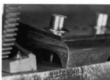
Fig. 6. Curved and polished outside edge of the comb bases, very unusual.
