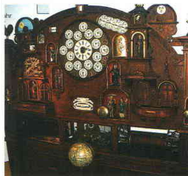
Fig. 18. Automated clock by Droll with astronomical features/organ/automata/religious figures.
