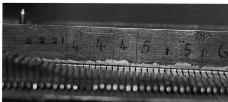
Fig. 4. Bass half of 5959 comb. Pairs of dots indicate g teeth, 192 and 384Hz. I added the numbers of teeth tuned to the same pitch, as indicated by the scribed pitch lines on the comb base.
