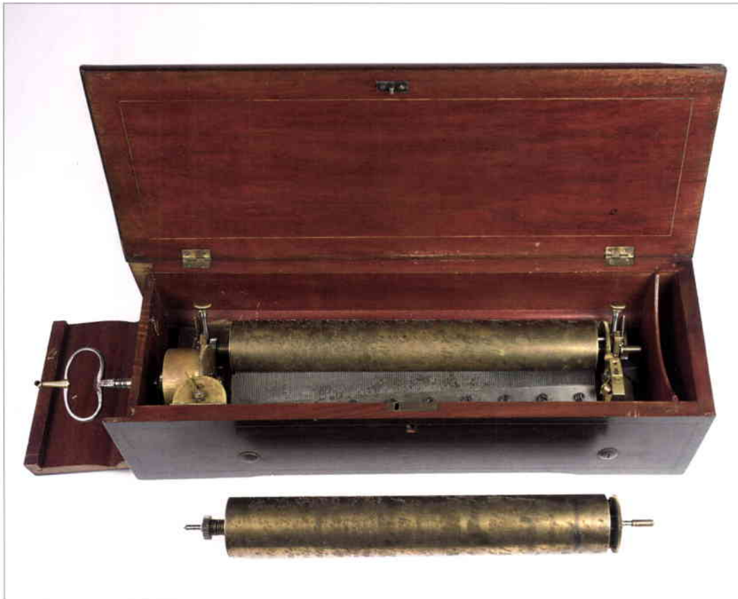
A mandoline changeable musical box by Lecoultré, with five cylinders each playing three airs.
