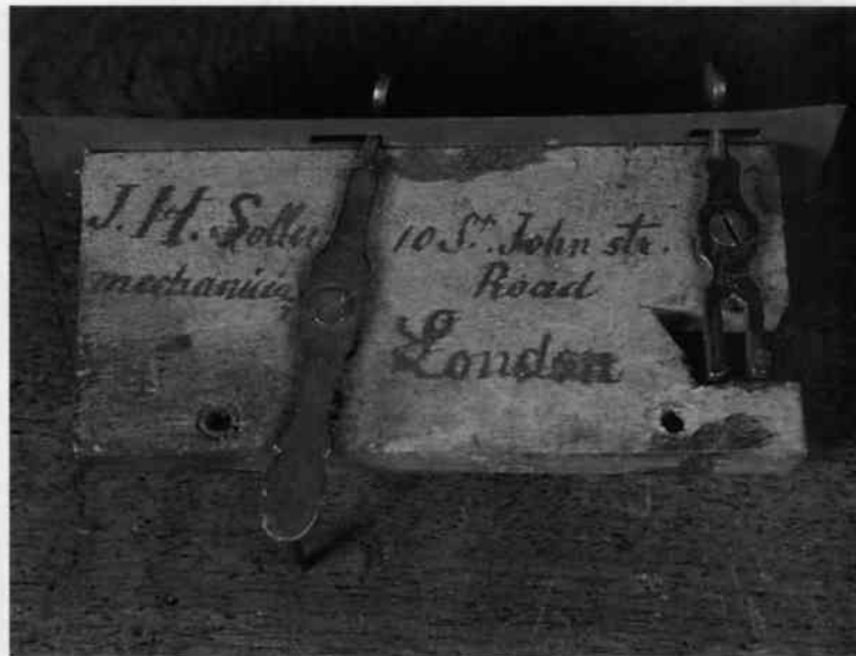
Fig. 14. A control panel of the early lever-wind period, with conventional slot in the change/repeat lever. St. John Street, London EC 1 is just north of Clerkenwell Road.
