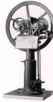
»Otto-Motor, 1877« Impressive tall exhibition model of world's first four-stroke engine, invented by N.A. Otto, Germany (8.2 ft. high)!
