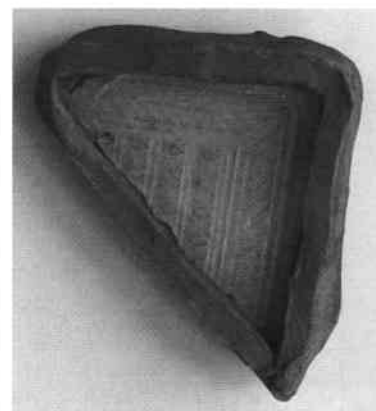
Fig. 8. The reverse side of the cover plate. When the Araldite-powder mix is hard, shape flat and remove shiny surface.
