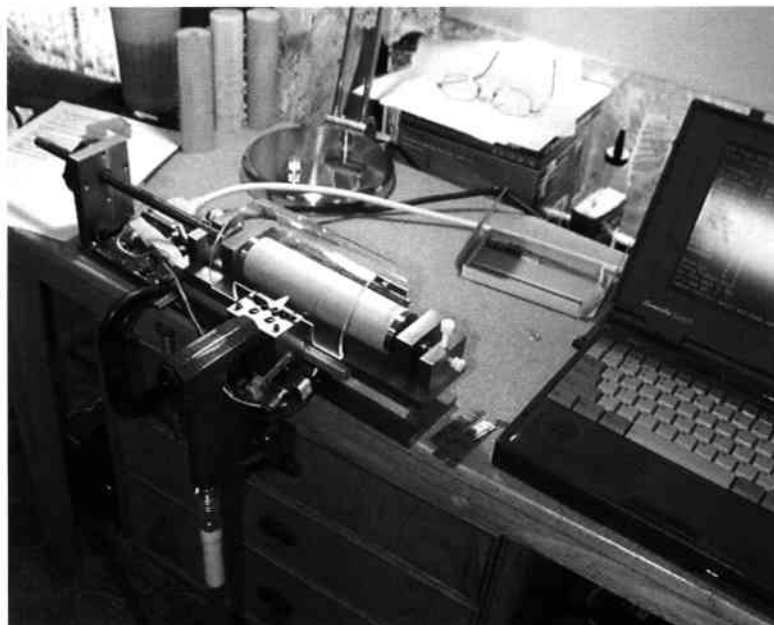
Fig. 10. A laptop computer controls the automatic pinner over a standard parallel port.
