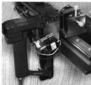
Fig. 8. The headless pinner can be fired automatically with a solenoid or triggered manually.
