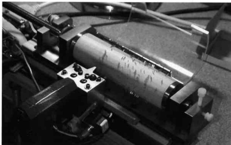
Fig. 6. A pneumatic "headless pinner" is used to install steel pins in the roller. as the blank roller is rotated, a lead screw advances the roller and mounting stage along a slide rail. This creates the one-tenth of an inch per revolution spiral path required for the pins.
