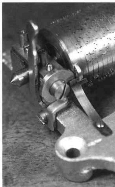
Fig. 14. Cylinder shoe holds the restraint spring clear of the tune change cam at the tune gap. The Change/Repeat lever is in Change position, with its lower member pulled away from the cam.
