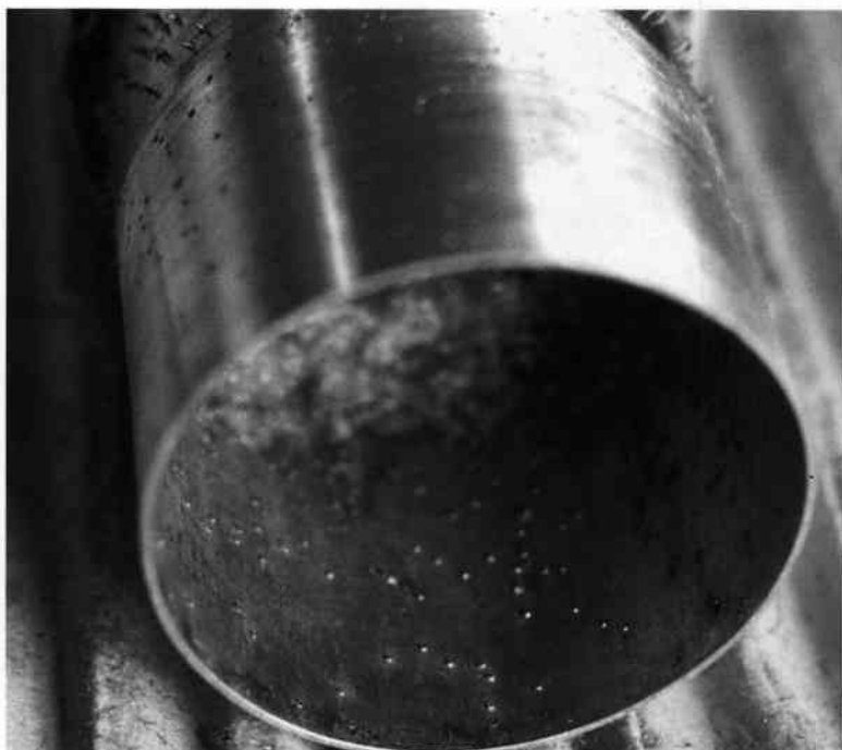
Fig. 10. View inside 37918 cylinder, showing how all the pin holes are lengthened.
