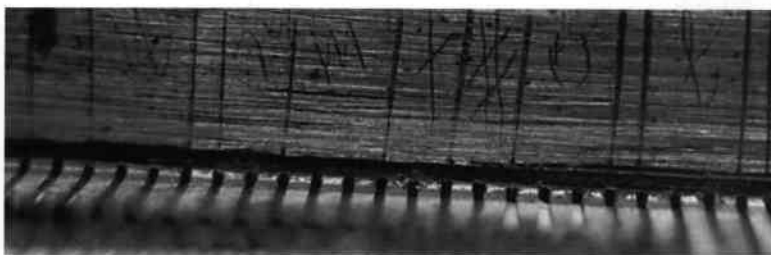
Fig. 3. Part of 37918 comb, pitch marks showing several groups of three teeth.
