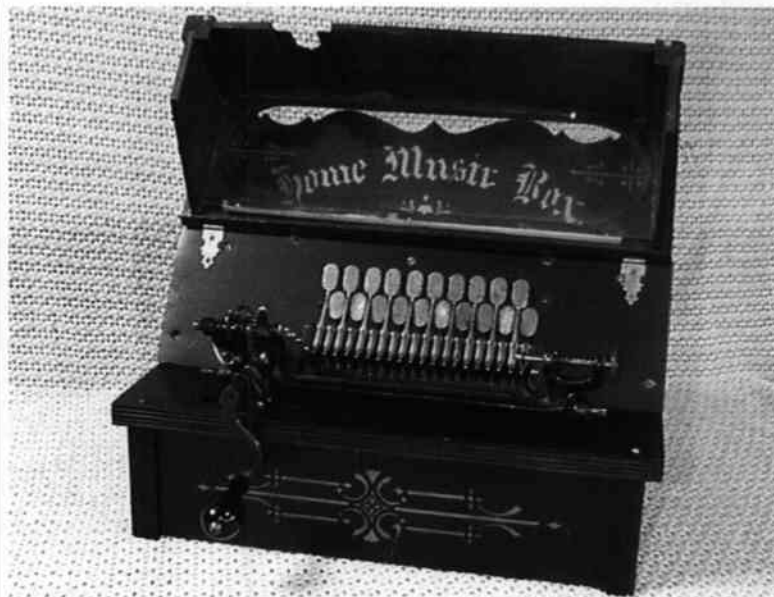
Fig. 2. The "Home Music Box" is the basic vacuum-operated model of the Gem Roller organ with a front cover and name board added for "show." Here the front cover is shown open revealing the double row of valves.
