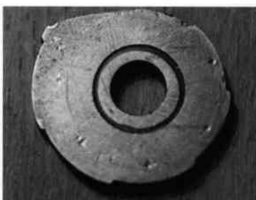
Fig. 12. Tune change cam. Dots mark the centre of each step. The drop from tune 6 to tune 1 is comparatively gradual.
