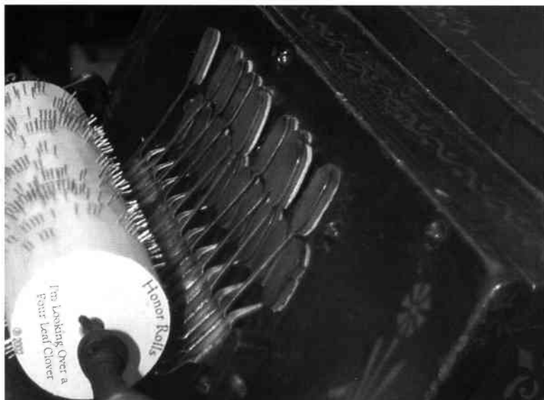
Fig. 3. The pins on the roller lift the valves to play the 20-note scale. The roller plays for about 40 seconds in three revolutions and then returns to the beginning.
