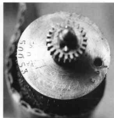
Fig. 4. Cylinder bass end stamped with the original maker's serial number 627, the "6" now drilled away, and new serial added, with scribed gamme number.
