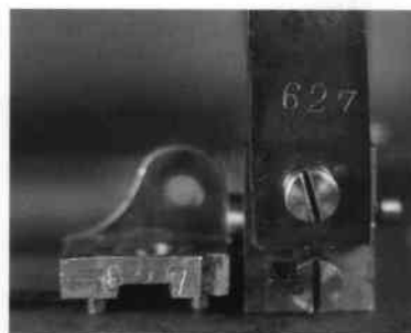
Fig. 6. Maker's serial 627 on governor and cylinder bearing.
