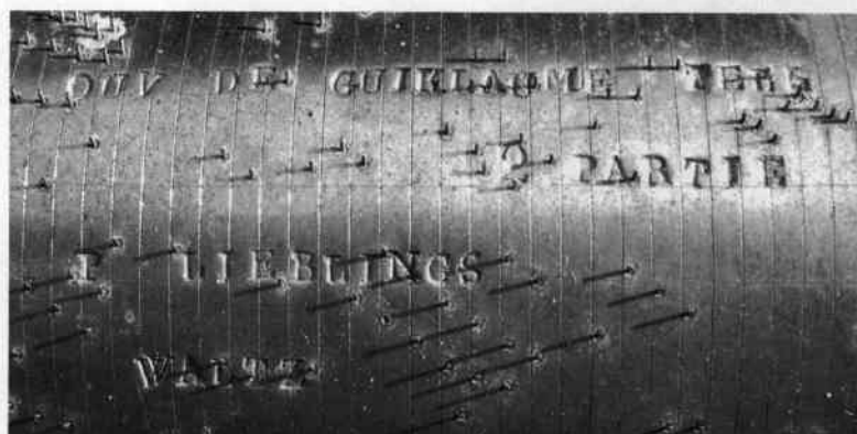
Fig. 8. Treble area of cylinder 12 stamped with its four tunes. The W. Tell overture is on two turns. The top and bottom serifs of the tune titles are so uniform that they were surely stamped while the brass sheet was flat.
