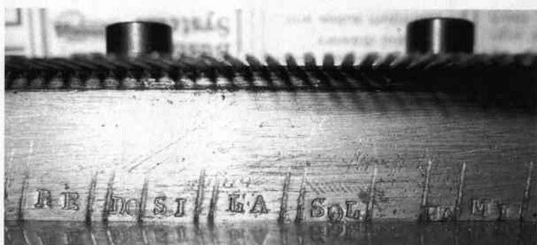
Fig. 9. Pitch notation stamped, with scribed lines at each pitch change, on serial 4826 comb.
