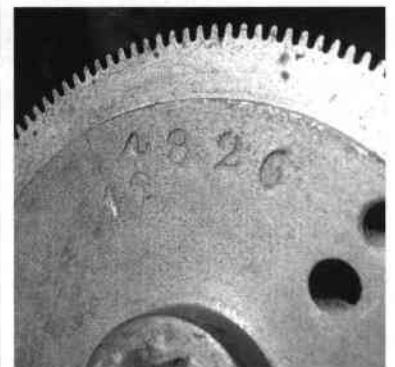
Fig. 6. Great wheel of cylinder no. 12 with its number stamped beside the serial number. The outer edge of the stop arm pin track is removed to allow free passage of the pin away from the wheel during cylinder change.
