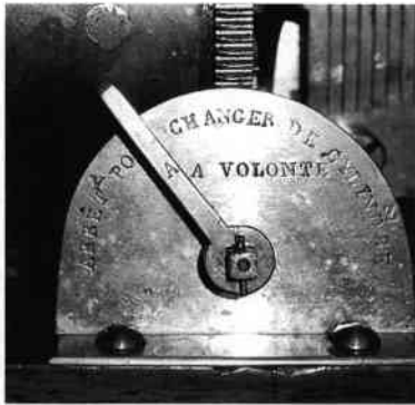
Fig. 3. The dial plate, screwed to the case front, showing lever A near point Y for "stop for change of cylinder." That locks the spring barrel. When turned to point Z it frees the spring and applies a locking bar to the bearing covers, see Fig. 12.
