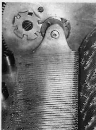
Fig. 10. Comb teeth detail. On the bass half of the comb, the hooked tips are bent up and the front half of each tooth is bent down, leaving all tips in their original straight line.
