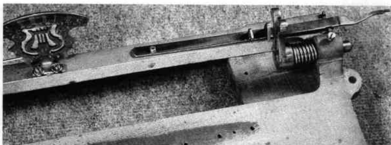
Fig. 3. Shows the control rod passing behind the tune indicator. A tension spring holds it towards the treble end. The cylinder slot is in the upright position, for changing cylinders. It slopes backwards to get the cylinder clear from the comb as soon as possible.
