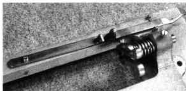
Fig. 4. Cylinder slot in playing position. It is held firmly in either position by the coil spring. The locating plate for the tune change lever is at back, right.
