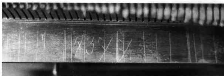
Fig. 8. Serial number and all pitch changes scribed on comb base.
