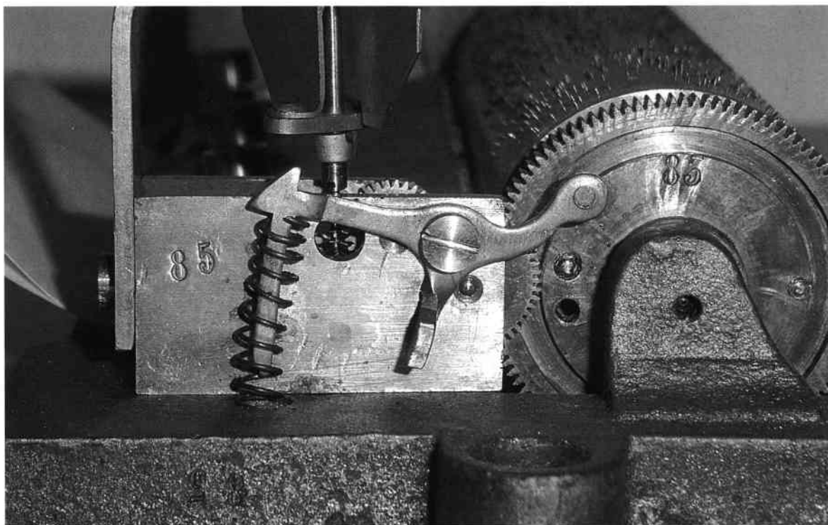
Fig. 7. Coil spring pushing the stop arm to STOP position. Blank 85 on governor and great wheel and, as usual, upside down on bedplate edge. No adjusting screw on governor.
