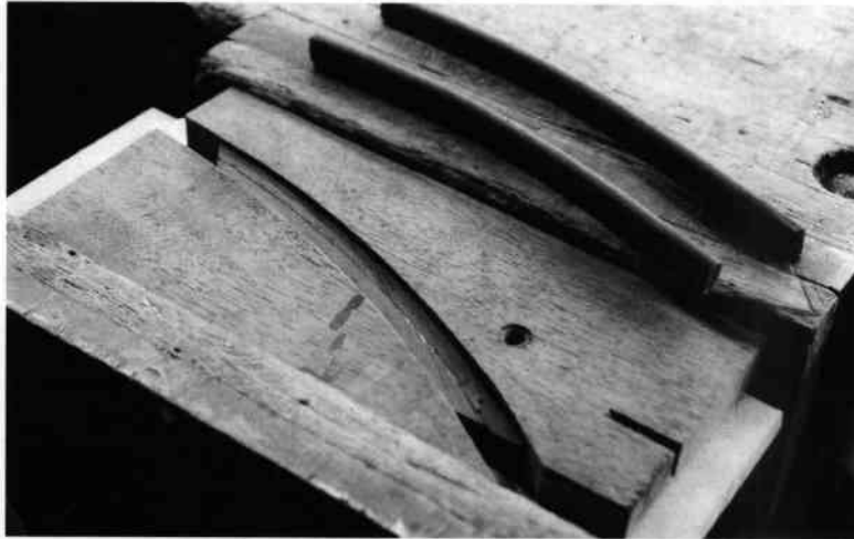
Fig. 2. Original parts clamped in the jig as the glue dries whilst new beads sit on the bench awaiting their trim.
