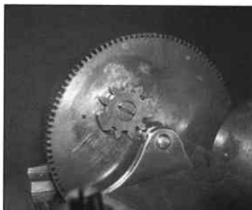
Fig. 5. Uncommon type of female stop, giving choice of four or five turns to wind up the spring. (Male peg awaiting restoration.)
