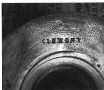
Fig.10. Clément's foundry marking on the cast brass spring cover of serial 43958.
